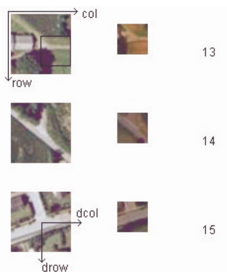
Fig. 2. Patches of the aerial image and the orthoimage. The matching gave the following results:
