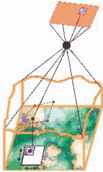
Fig. 1. Matching between patches of an aerial image and the existing orthoimage is used to georeference the new aerial image. At the position of best-fit spatial (XYZ-) coordinates can be derived from the orthoimage and the height model. Together with coordinates of the image patch centre they serve as input to a bundle adjustment which derives the outer orientation of the aerial image. With these parameters (spatial coordinates of the perspective centre and the spatial position of the camera axis) an aerial image is georeferenced.
